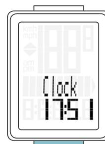
Press the **SET button** to confirm the hour setting.
