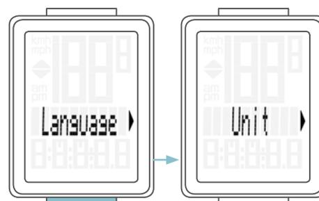
Press the **SET button** to open the unit setting.
