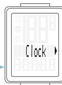
Press the **SET button** to open the setting for the clock.
