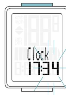
Press the **SET button** to confirm the minute setting.
